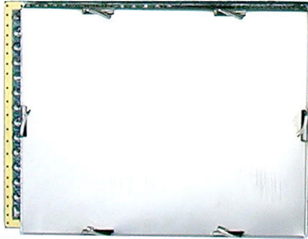
LPD-24RC Transceiver Module Top Side Shield Installed:
