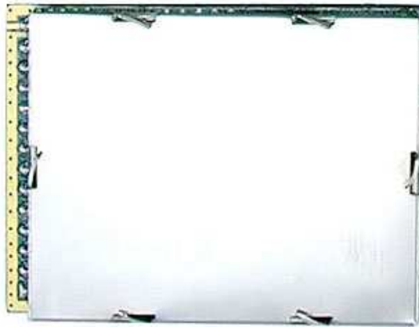
6.1 HPD-24RC Transceiver Module Top Side with Shield Installed:
