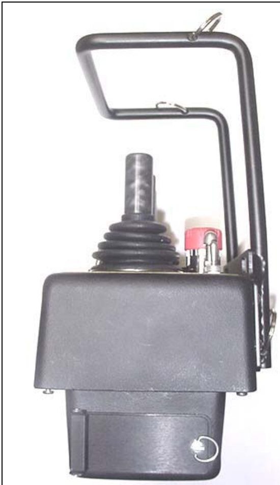
Left Side of T42 Radio Remote Control Console
