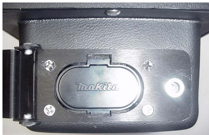
Ni-Cd Battery Pack installed in T42
