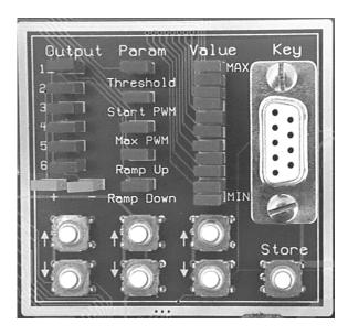
To enable the configuration panel, plug in the user configuration key supplied. The display will initially be displaying "Output" 1 + , no "Param" lights will be illuminated, and the "Value" lights will be displaying the Start PWM and MAX PWM as solid lights, and the actual speed output as a flashing light. The flashing light will move as the speed dial on the transmitter is rotated. You will also see the green light next to the 1+ output go brighter and dimmer.
