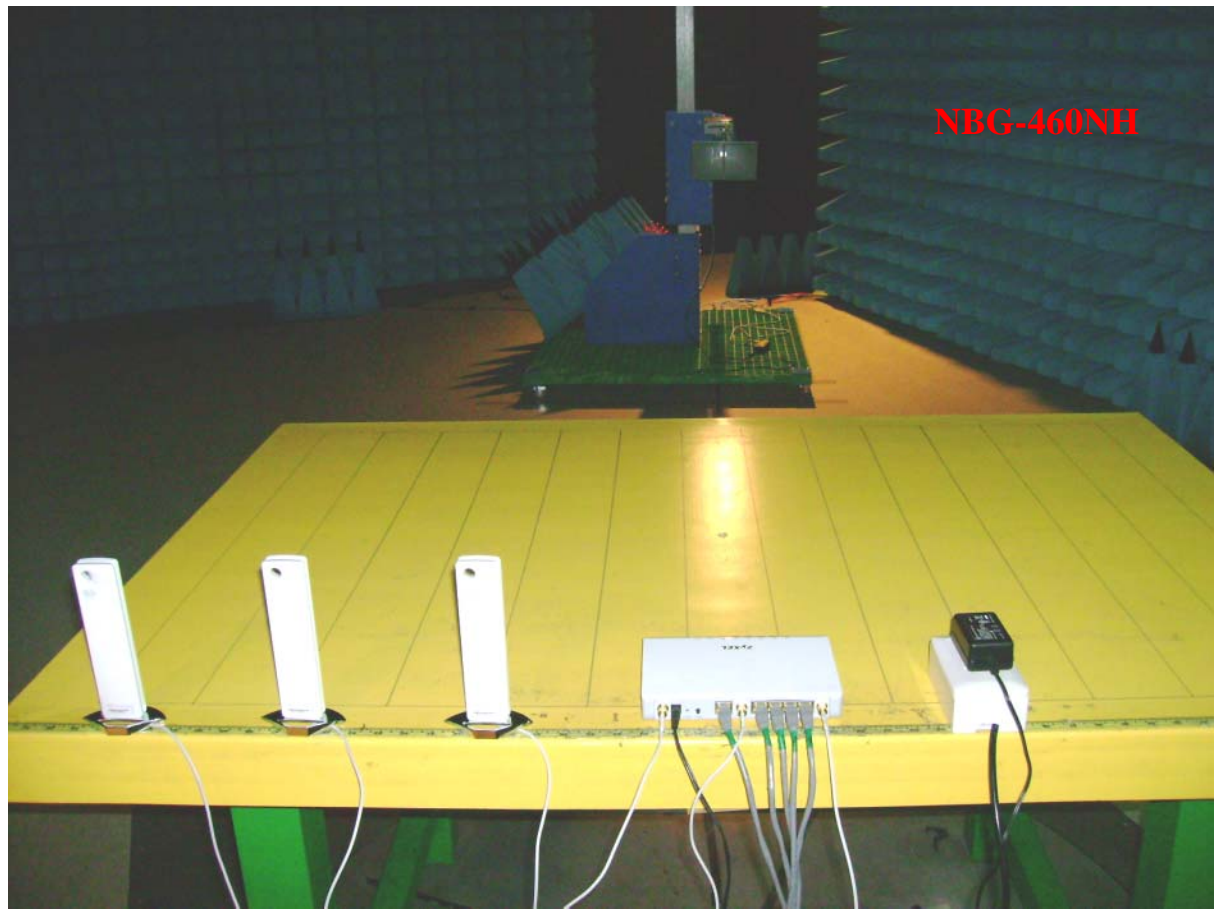
Photo 2: Radiated Emission Test set-up photo
