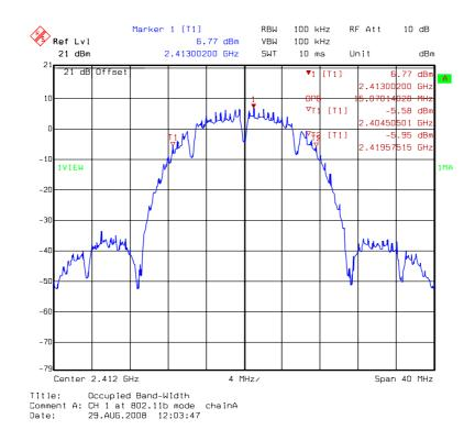
Chain A: 99% Occupied Bandwidth @ 802.11b mode channel 6
