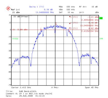
Chain C: 6dB Bandwidth @ 802.11b mode channel 6
