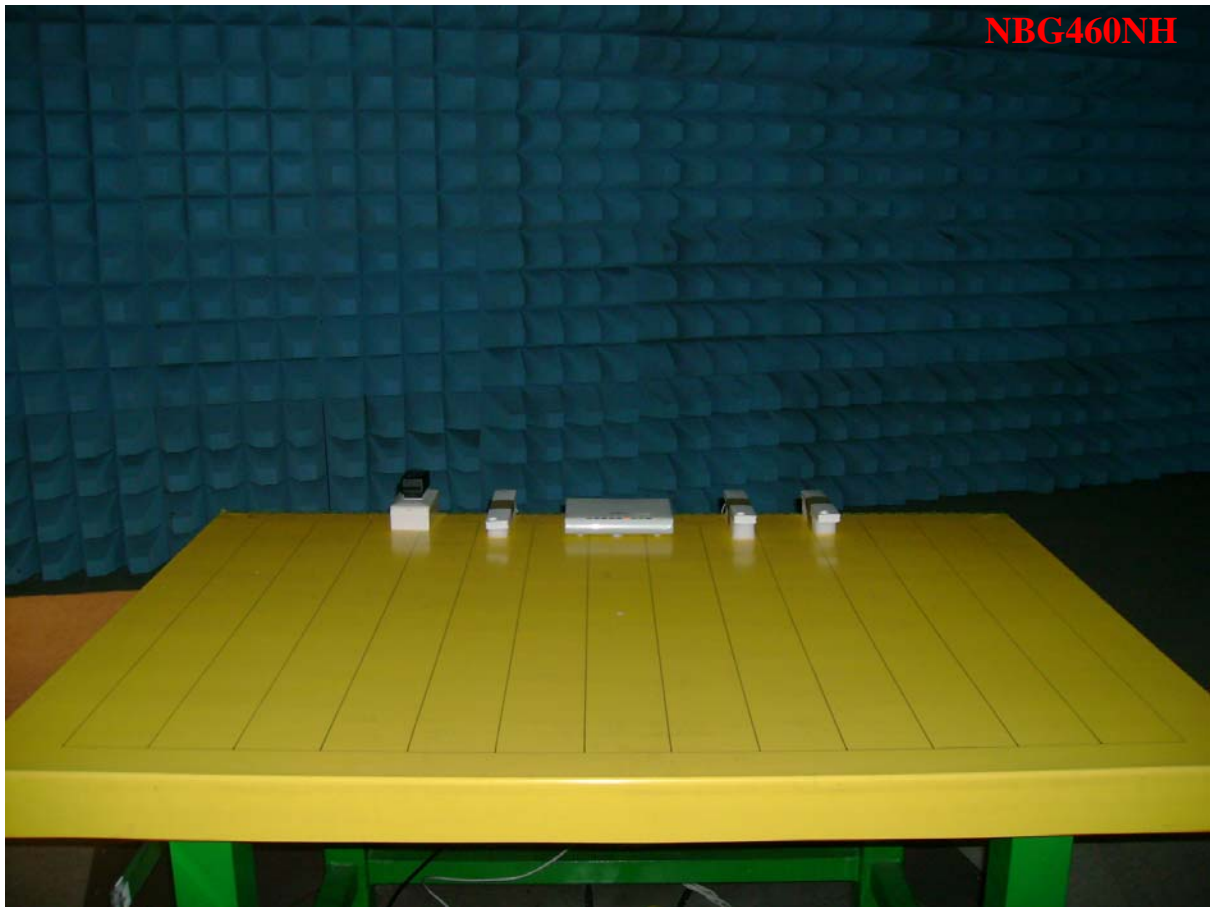
Photo 1: Radiated Emission Test set-up photo
