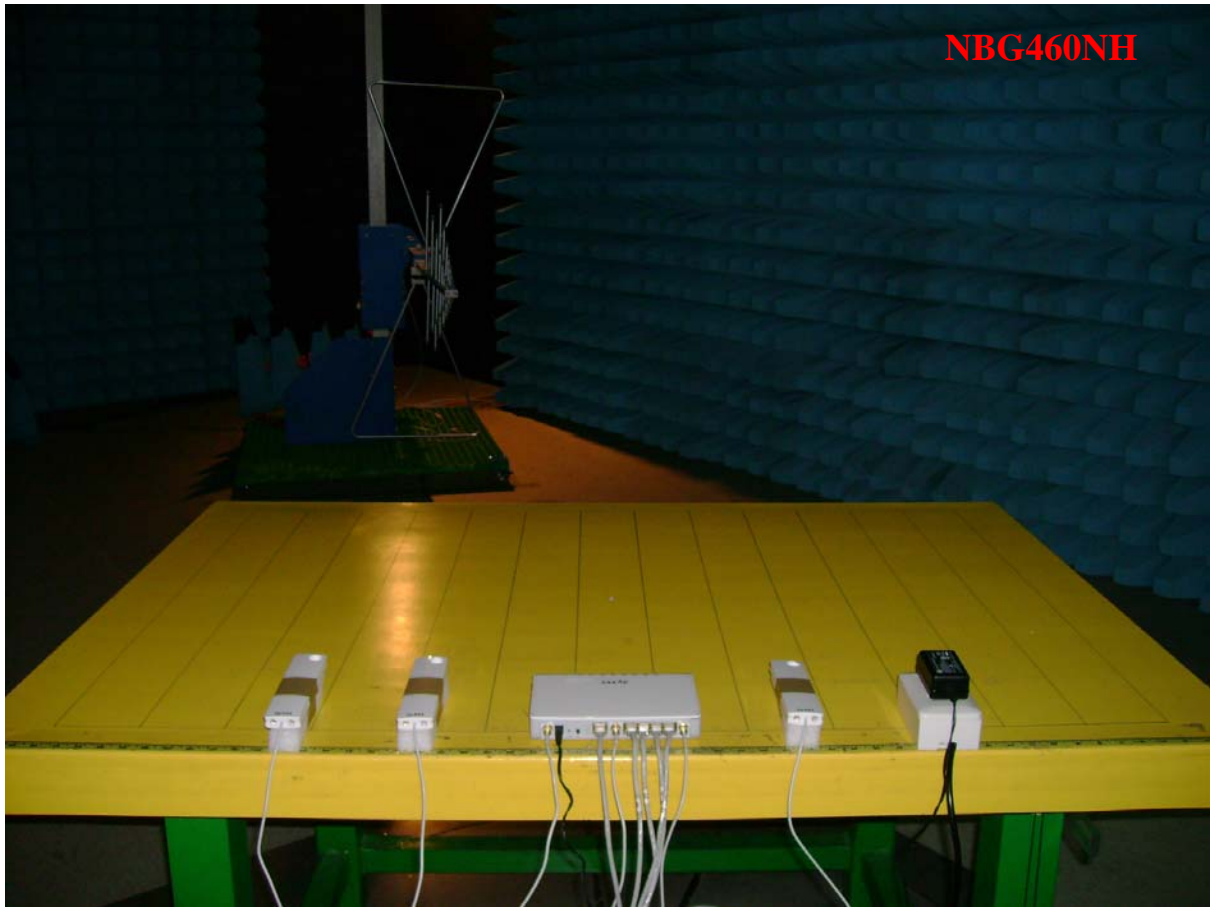
Photo 2: Radiated Emission Test set-up photo
