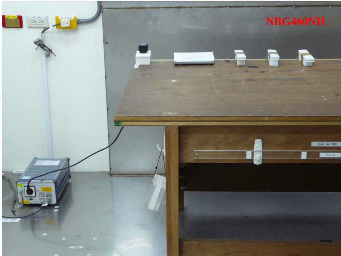
Photo 1: Conducted Emission Test Set-up photo
