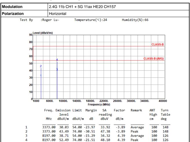
Note 1: Emission Level (dBuV/m) = SA Reading (dBuV/m) + Factor\* (dB/m)
