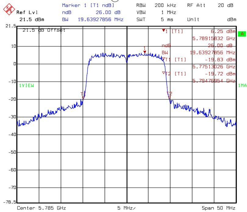
**Chain 1: 26 dB Bandwidth @ 802.11n HT20 mode channel 161**
