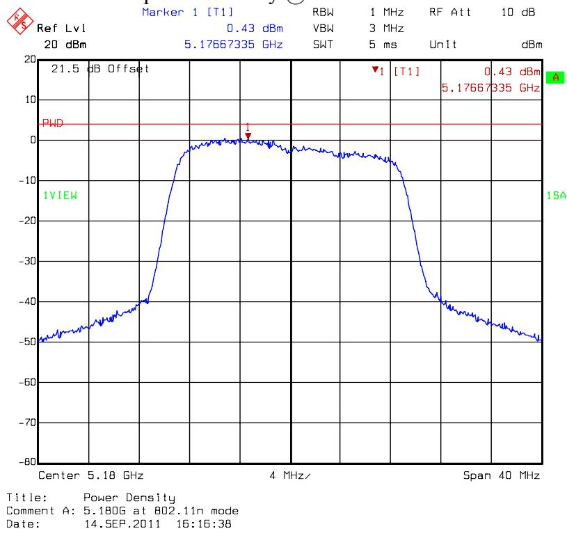
**Chain 1: Power Spectral Density @ 802.11n HT20 mode channel 40**
