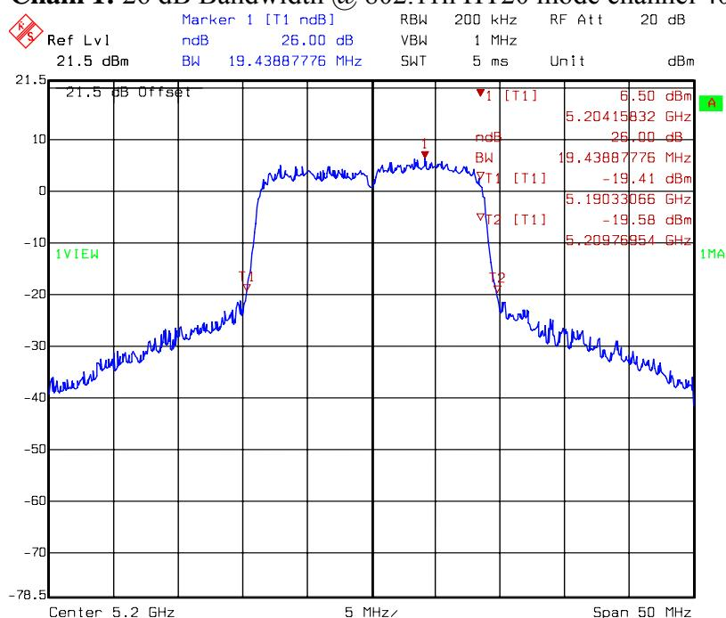
**Chain 1: 26 dB Bandwidth @ 802.11n HT20 mode channel 48**
