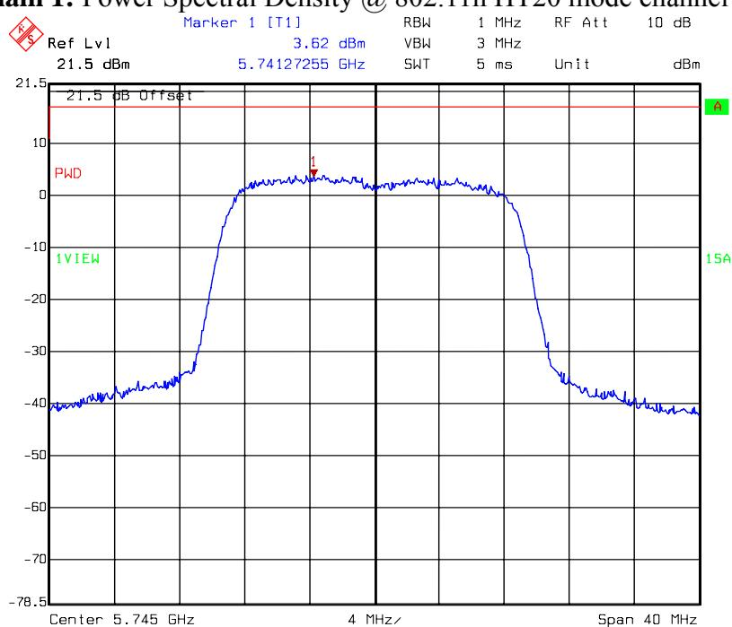
**Chain 1: Power Spectral Density @ 802.11n HT20 mode channel 157**
