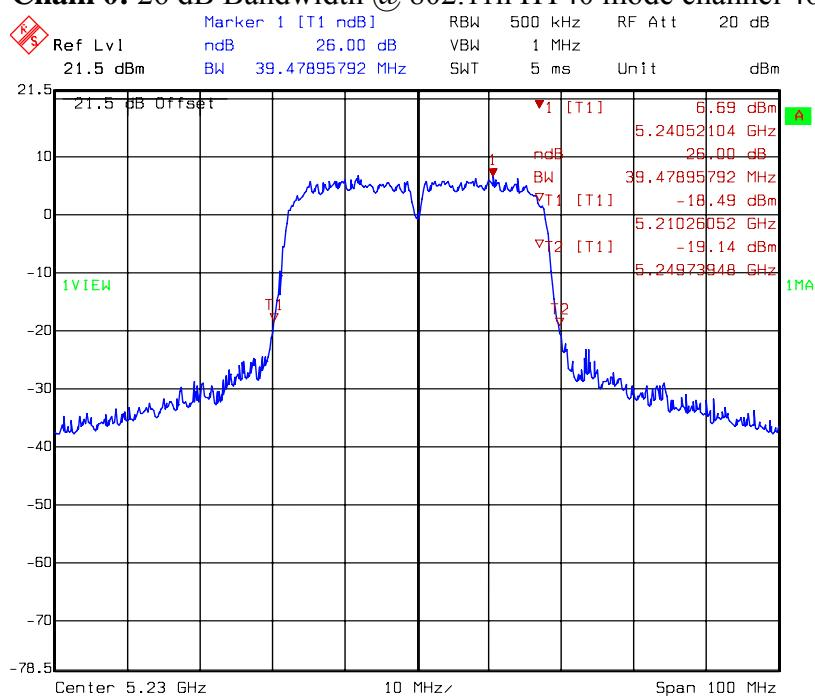
**Chain 0:** 26 dB Bandwidth @ 802.11n HT40 mode channel 151
