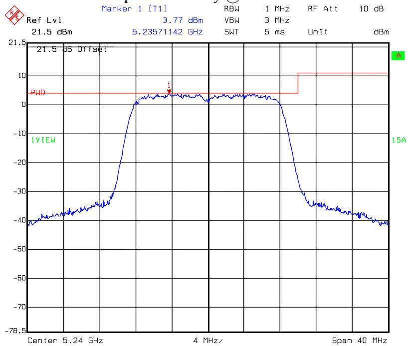
**Chain 1: Power Spectral Density @ 802.11a mode channel 149**
