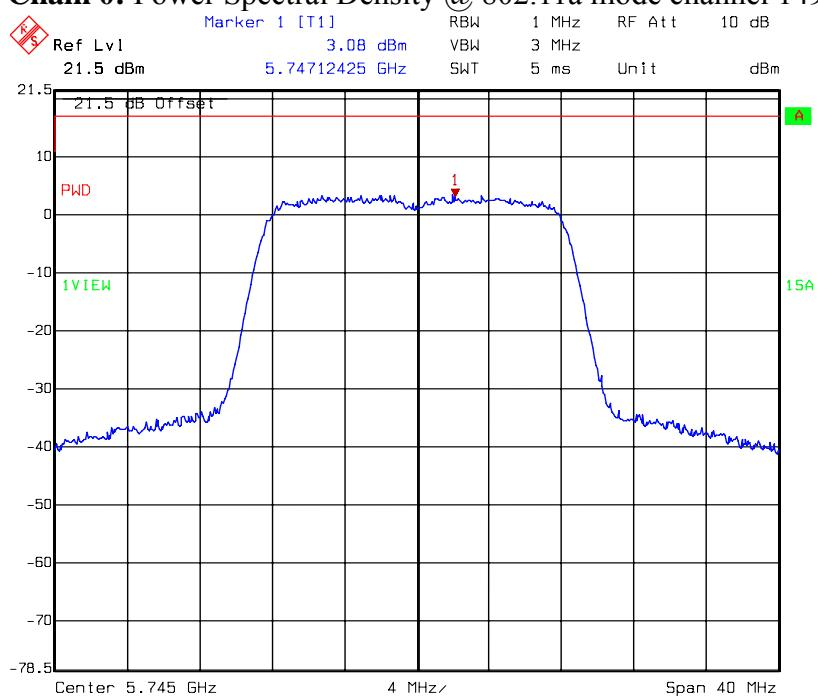
**Chain 0: Power Spectral Density @ 802.11a mode channel 157**
