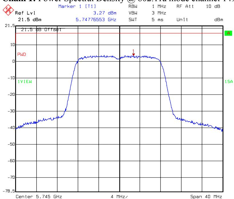
**Chain 1: Power Spectral Density @ 802.11a mode channel 157**
