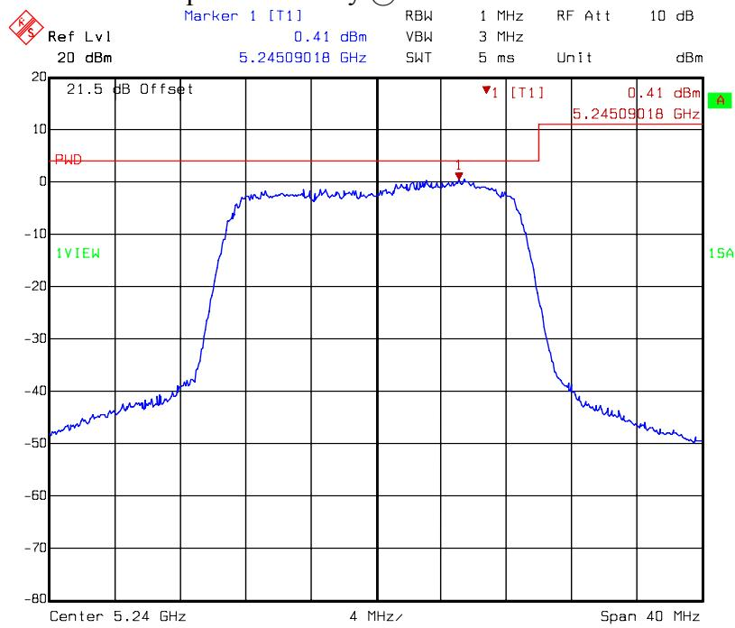
**Chain 1: Power Spectral Density @ 802.11n HT20 mode channel 149**
