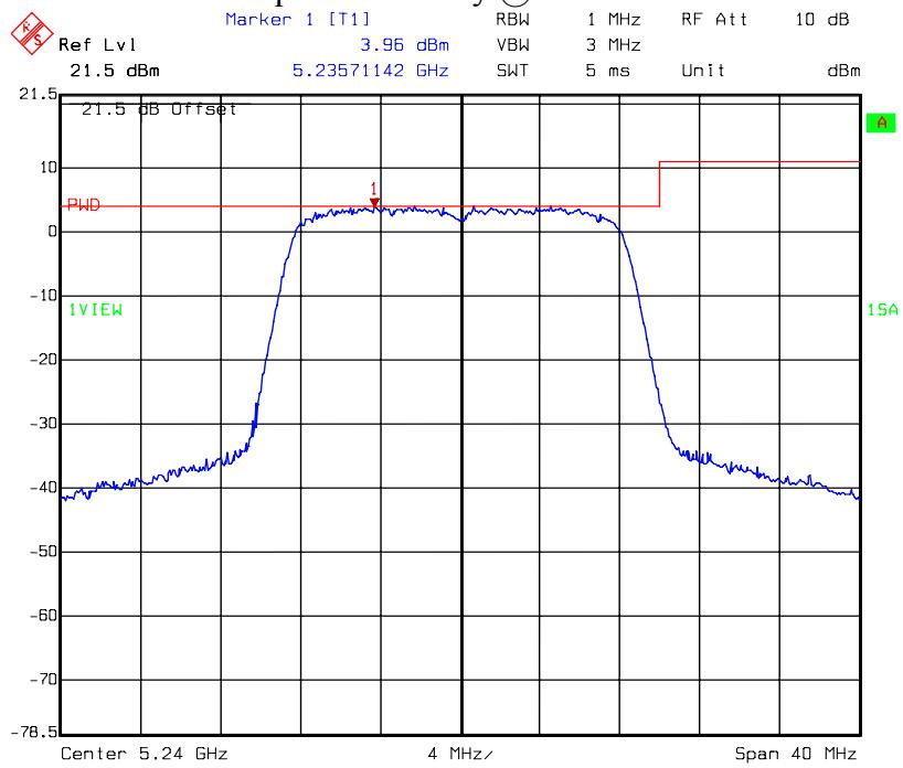
**Chain 0: Power Spectral Density @ 802.11a mode channel 149**
