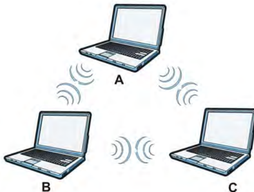
Figure 196 Peer-to-Peer Communication in an Ad-hoc Network
