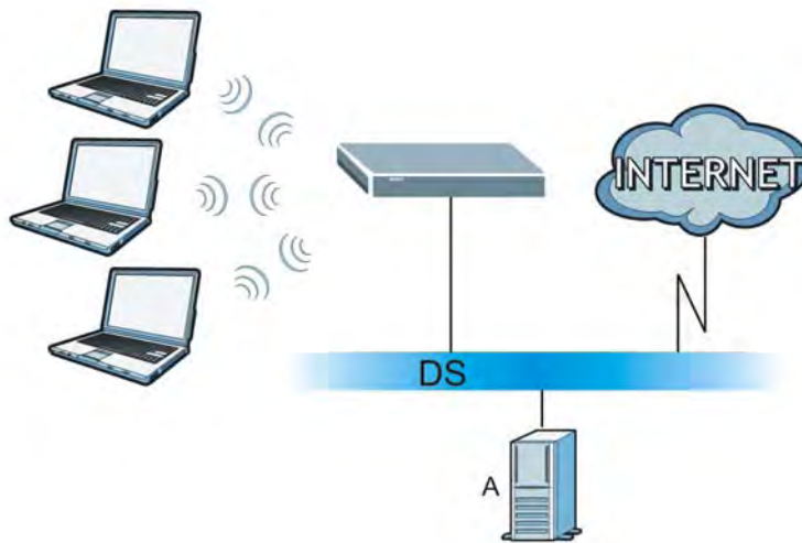
Figure 200 WPA(2) with RADIUS Application Example
