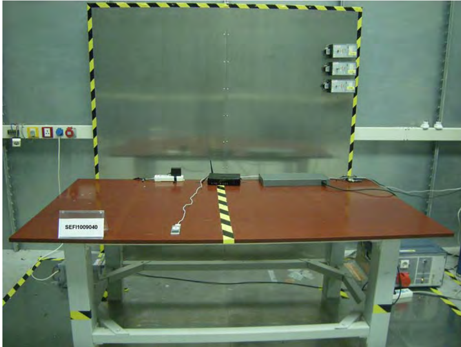
Front View of Conducted Emission Test
