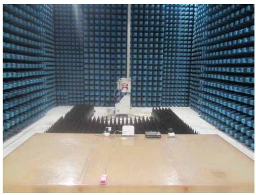
Test Mode: Transmitting Description: Front View of Radiated Emission Test Setup for Above 18GHz
