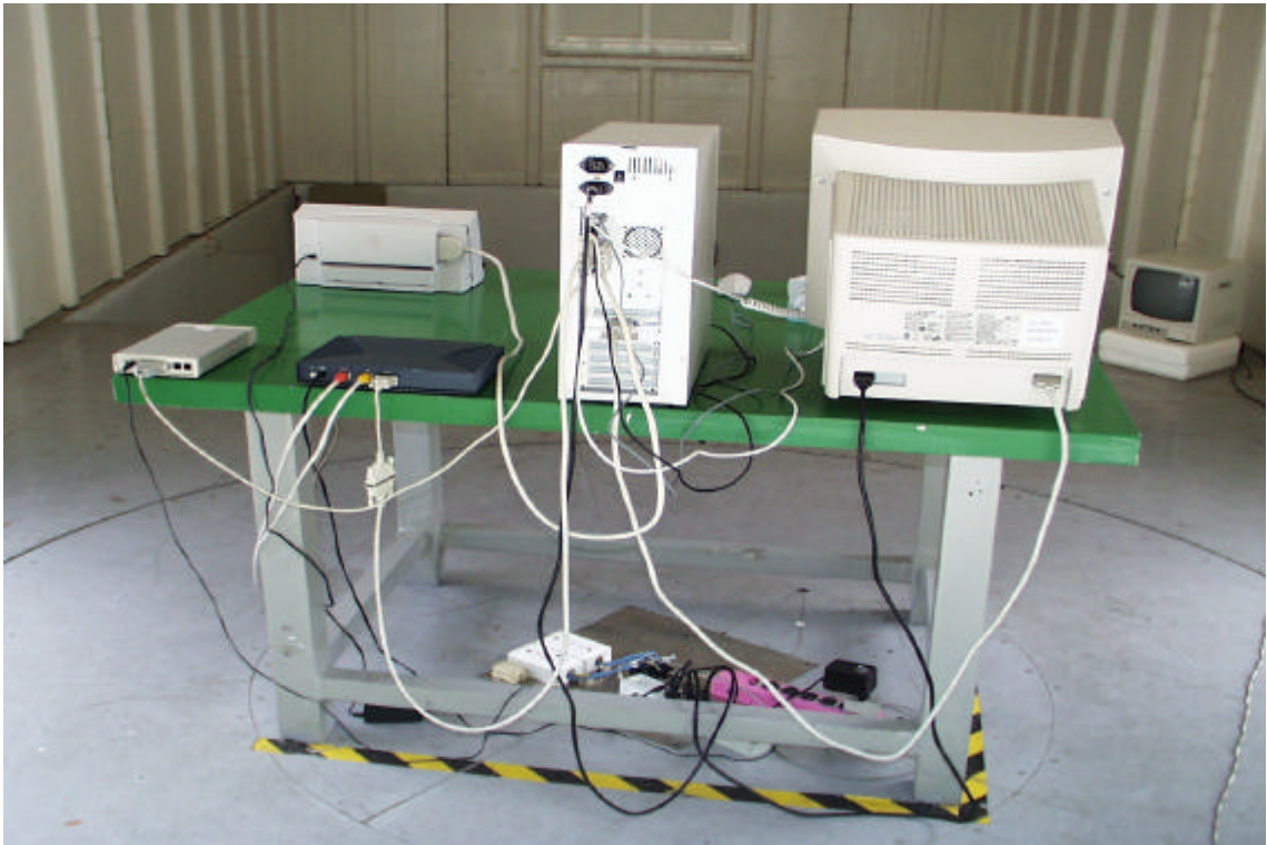
Back View of Conducted Test ( Mode 1)
