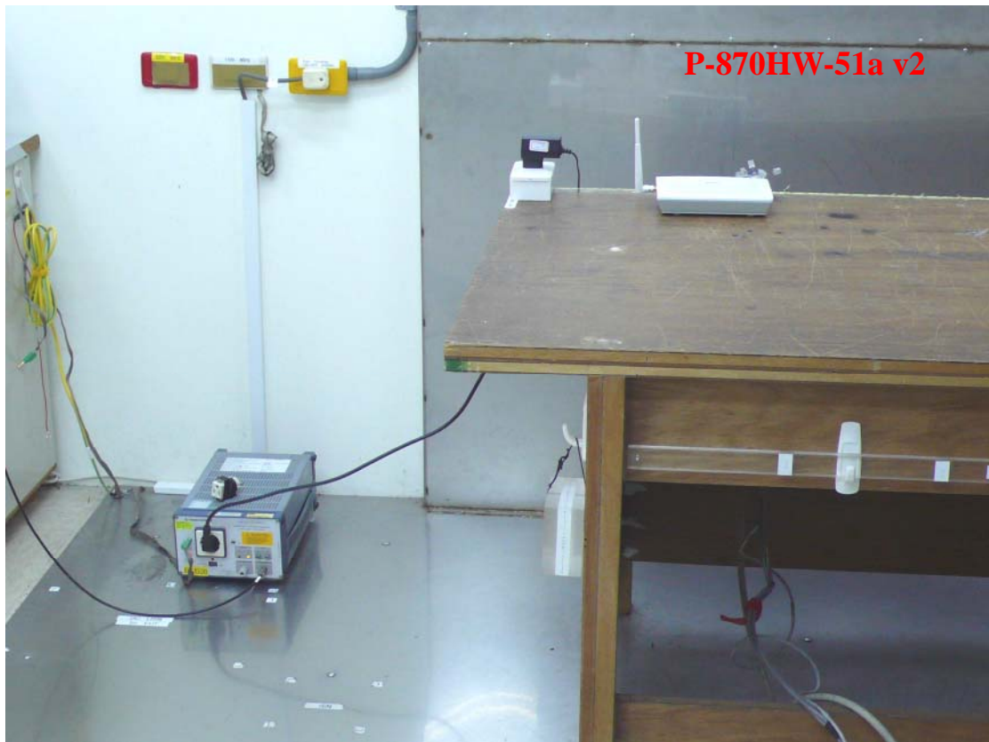
Photo 1: Conducted Emission Test Set-up photo
