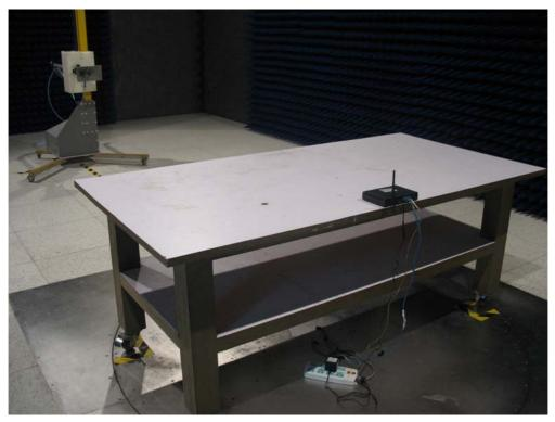
Test Mode: Mode 2: Transmit by 802.11gDescription: Front View of Radiated Emission Test Setup for Under 1GHz
