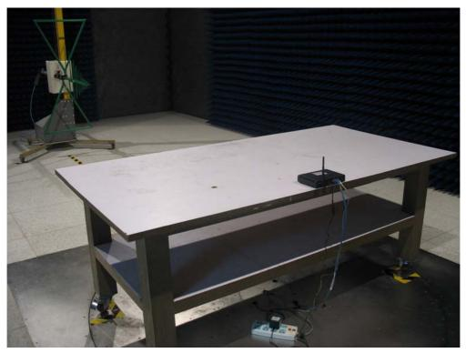
Test Mode : Mode 1: Transmit by 802.11b Description : Front View of Radiated Emission Test Setup for Above 1GHz
