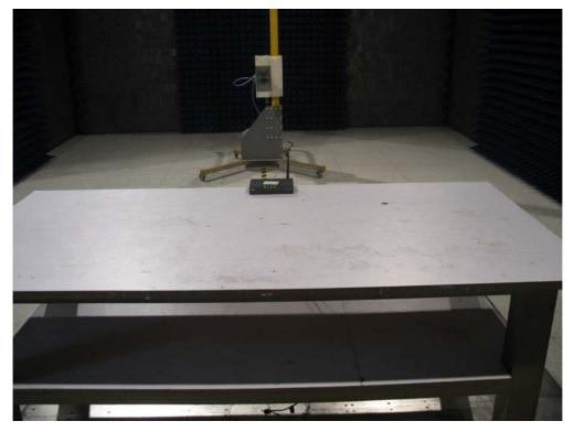
Test Mode: Mode 2: Transmit by 802.11gDescription: Back View of Radiated Emission Test Setup for Above 1GHz
