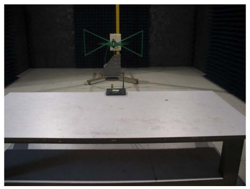
Test Mode: Mode 2: Transmit by 802.11gDescription: Back View of Radiated Emission Test Setup for Under 1GHz
