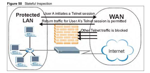
The previous figure shows the Prestige's default firewall rules in action as well as demonstrates how stateful inspection works. User A can initiate a Telnet session from within the LAN and responses to this request are allowed. However other Telnet traffic initiated from the WAN is blocked.
