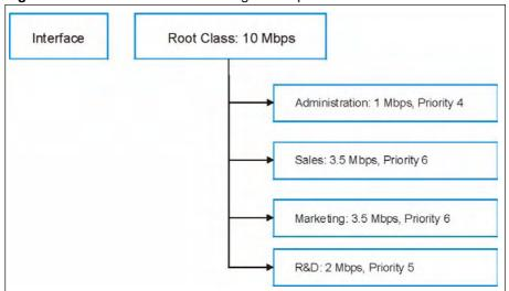
Figure 91 Maximize Bandwidth Usage Example
