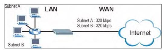
Figure 88 Subnet-based Bandwidth Management Example
