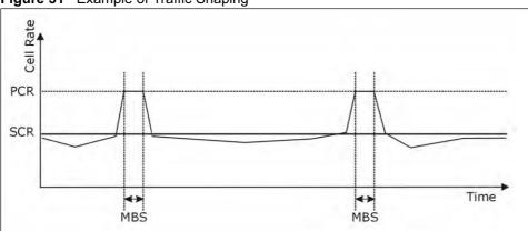
Figure 31 Example of Traffic Shaping
