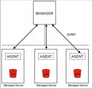
An SNMP managed network consists of two main components: agents and a manager.
