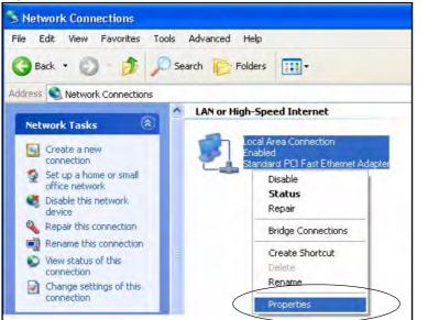
Figure 238 Windows XP: Control Panel: Network Connections: Properties
