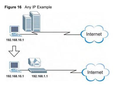
The Any IP feature does not apply to a computer using either a dynamic IP address or a static IP address that is in the same subnet as the Prestige's IP address.
