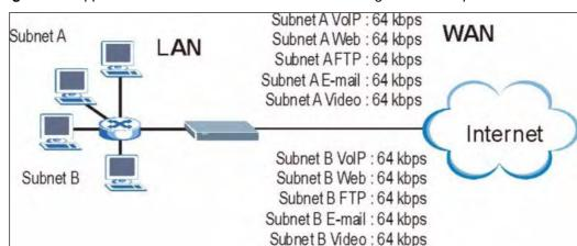
Figure 89 Application and Subnet-based Bandwidth Management Example
