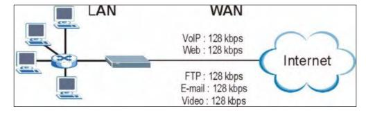
Figure 87 Application-based Bandwidth Management Example
