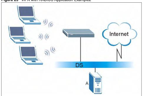
Figure 23 WPA with RADIUS Application Example2
