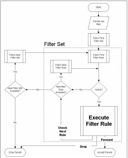
You can apply up to four filter sets to a particular port to block various types of packets. Because each filter set can have up to six rules, you can have a maximum of 24 rules active for a single port.
