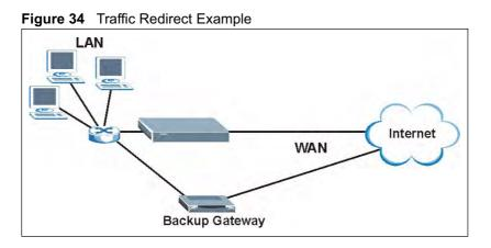
The following network topology allows you to avoid triangle route security issues when the backup gateway is connected to the LAN. Use IP alias to configure the LAN into two or three logical networks with the Prestige itself as the gateway for each LAN network. Put the protected LAN in one subnet (Subnet 1 in the following figure) and the backup gateway in another subnet (Subnet 2). Configure filters that allow packets from the protected LAN (Subnet 1) to the backup gateway (Subnet 2).
