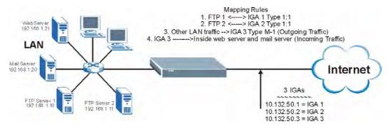
In this case you need to configure Address Mapping Set 1 from Menu 15.1 - Address Mapping Sets. Therefore you must choose the Full Feature option from the Network Address Translation field (in menu 4 or menu 11.3) inFigure 156 on page 265.
