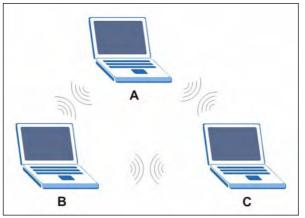
Figure 265 Peer-to-Peer Communication in an Ad-hoc Network
