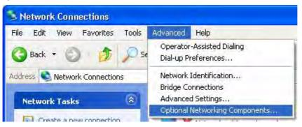
**4** The Windows Optional Networking Components Wizard window displays. Select Networking Service in the Components selection box and click Details.
