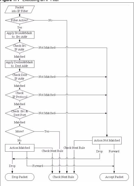
Figure 171 Executing an IP Filter
