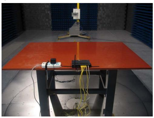
Test Mode: Mode 2: Transmitter by 802.11g
