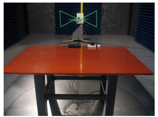
Test Mode: Mode 1: Transmitter by 802.11b
