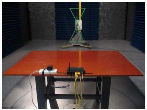
Test Mode: Mode 1: Transmitter by 802.11b
