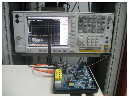
Test Mode: Mode 2: Transmitter by 802.11g
