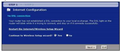
If the wizard still cannot detect a connection type and the following screen appears (see Figure 18 on page 58), click **Next** and refer to Section 3.2.2 on page 58 on how to configure the ZyXEL Device for Internet access manually.
