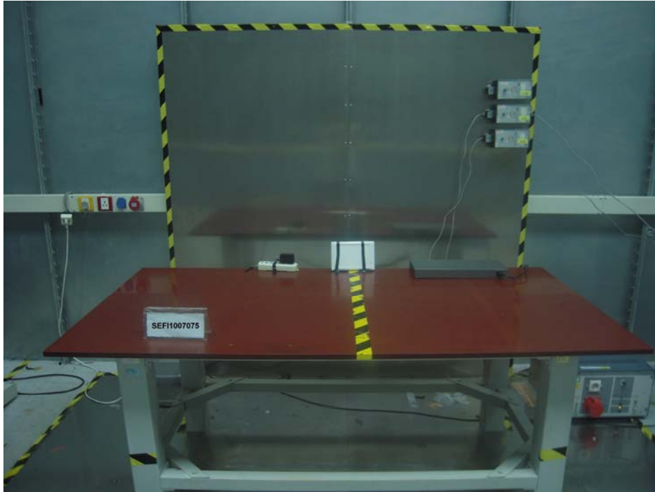
Front View of Conducted Emission Test
