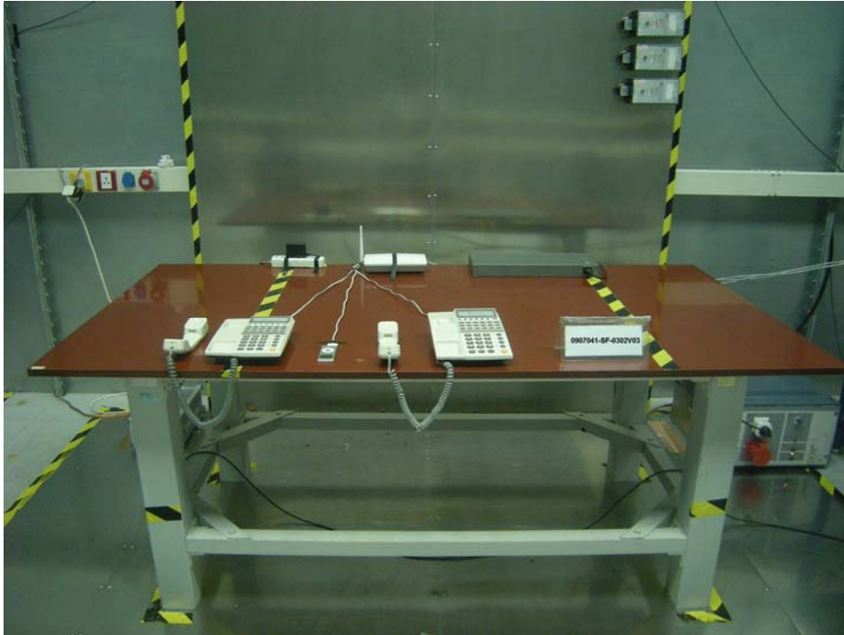
Front View of Conducted Emission Test
