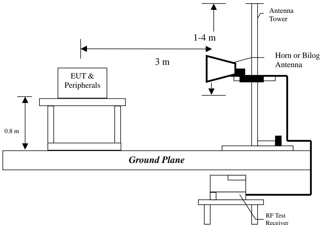
The frequency range from 30MHz to 1000MHz using Bilog Antenna.
