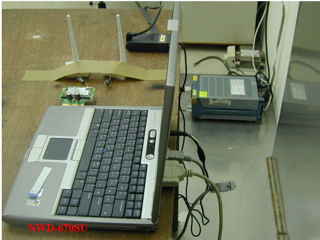
Photo 3: Conducted Emission Test Set-up photo
