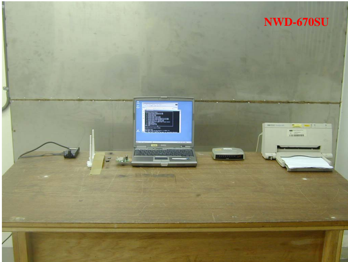
Photo 1: Conducted Emission Test Set-up photo
