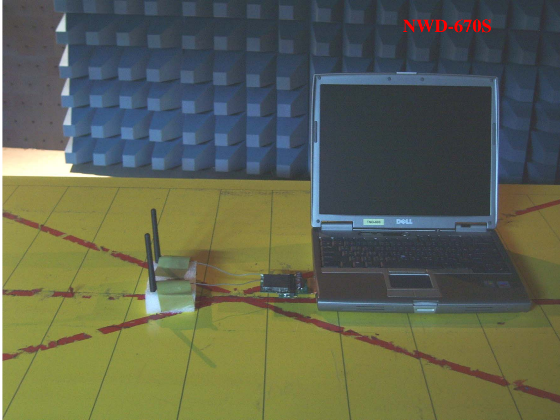
Photo 1: Radiated Emission Test Set-up
