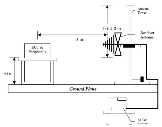
Radiated emissions were invested cover the frequency range from 30MHz to 1000MHz using a receiver RBW of 120kHz record QP reading, and the frequency over 1GHz using a spectrum analyzer RBW of 1MHz and 10Hz VBW record Average reading. (15.209 paragraph), the Peak reading (1MHz RBW/VBW) recorded also on the report.
