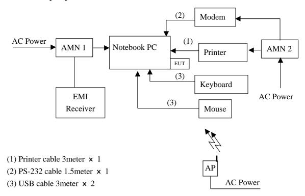
The EUT are connected to the main power through a line impedance stabilization network (LISN). This provides a 50 ohm/50uH coupling impedance for the measuring equipment. The peripheral devices are also connected to the main power through a LISN that provides a 50ohm/50uH coupling impedance with 50ohm termination.
