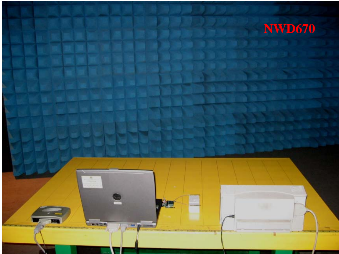
Photo 2: Radiated Emission Test set-up photo
