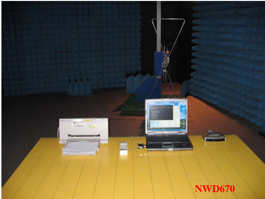
Photo 1: Radiated Emission Test set-up photo
