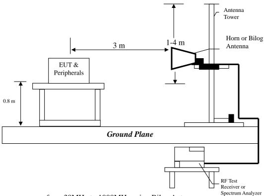
The frequency range from 30MHz to 1000MHz using Bilog Antenna. The frequency range over 1GHz using Horn Antenna.
