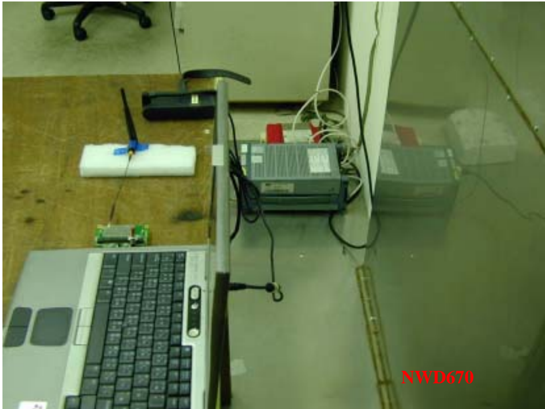
Photo 2: Conducted Emission Test Set-up photo
