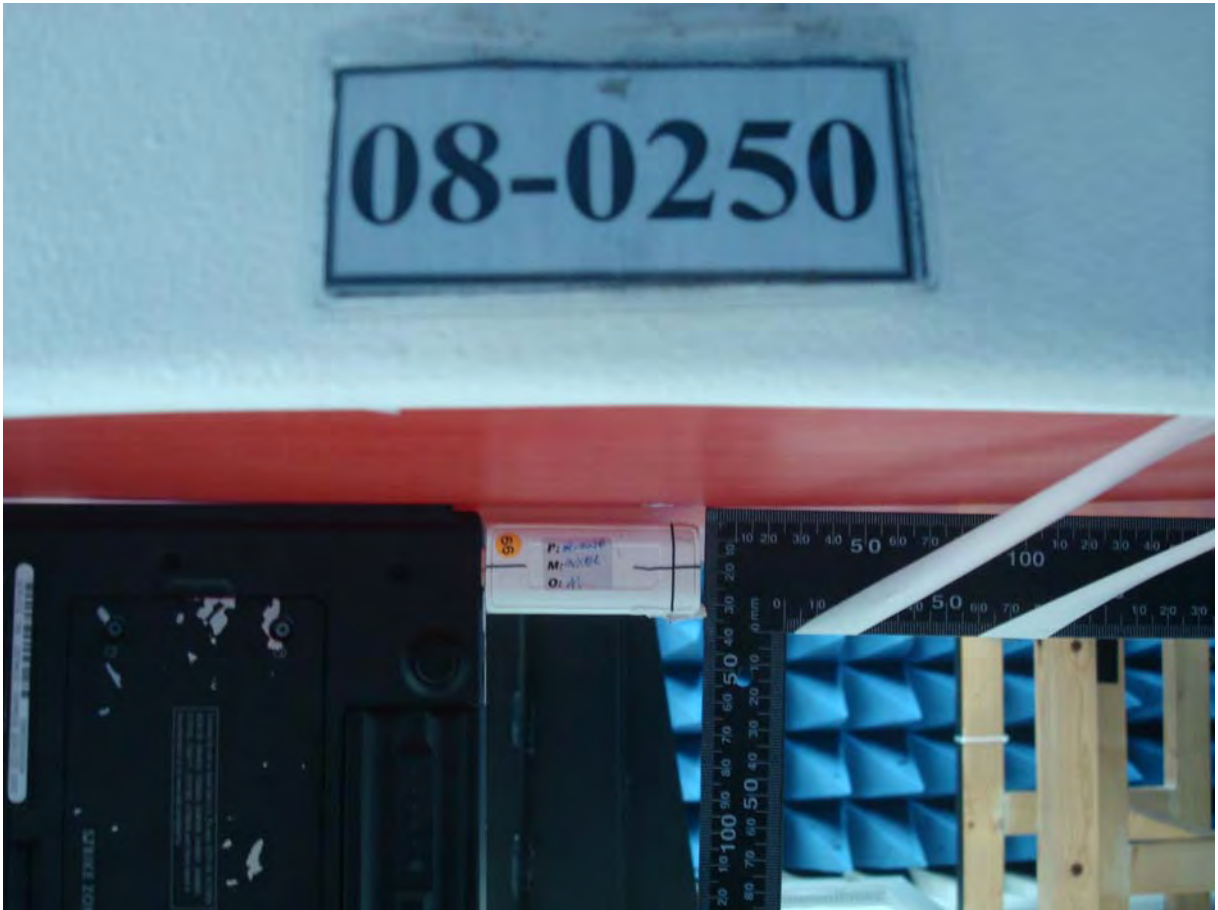
Figure 16. Body SAR Test Setup (Flat Section)
