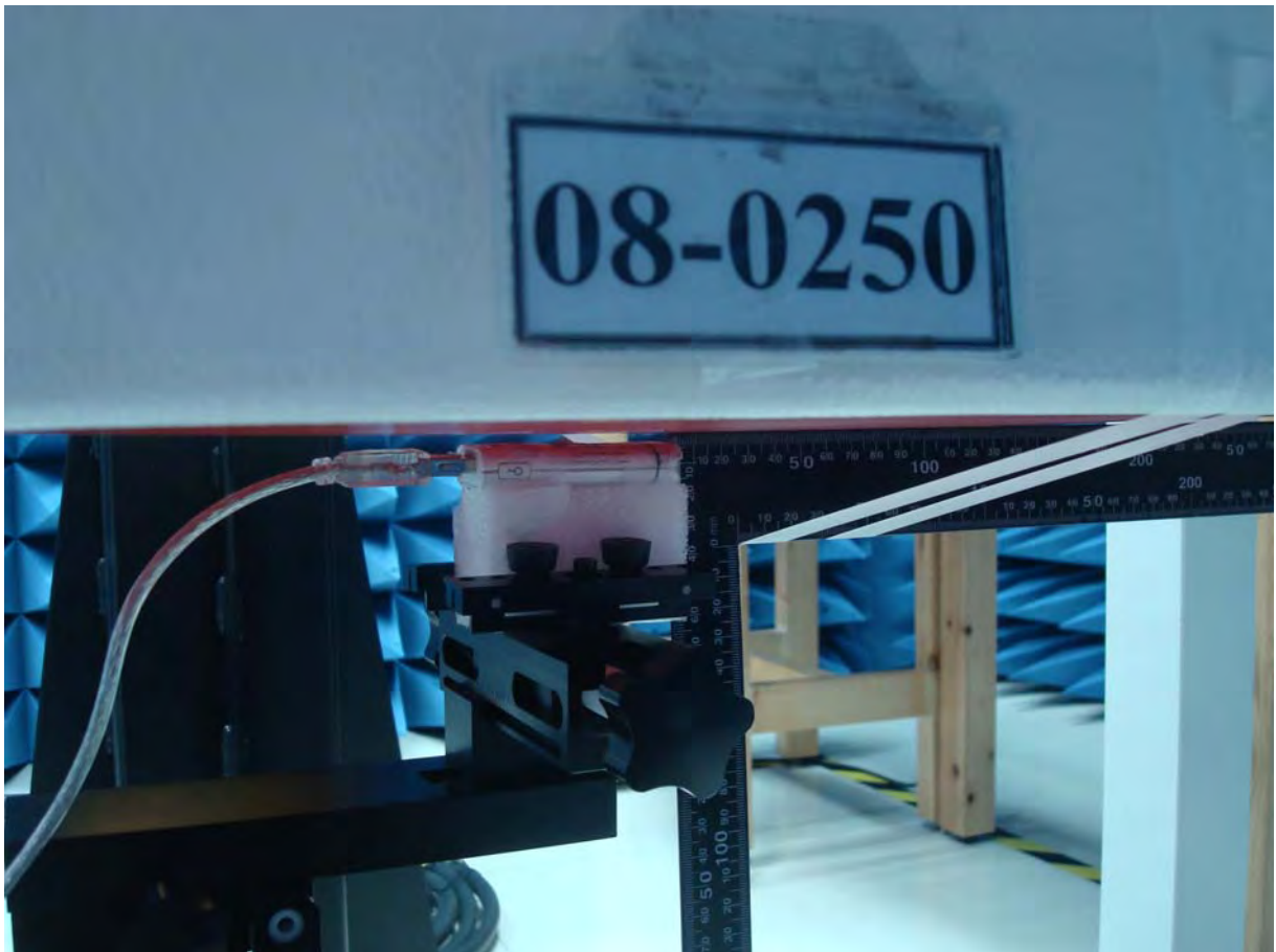
Figure 14. Body SAR Test Setup (Flat Section)
