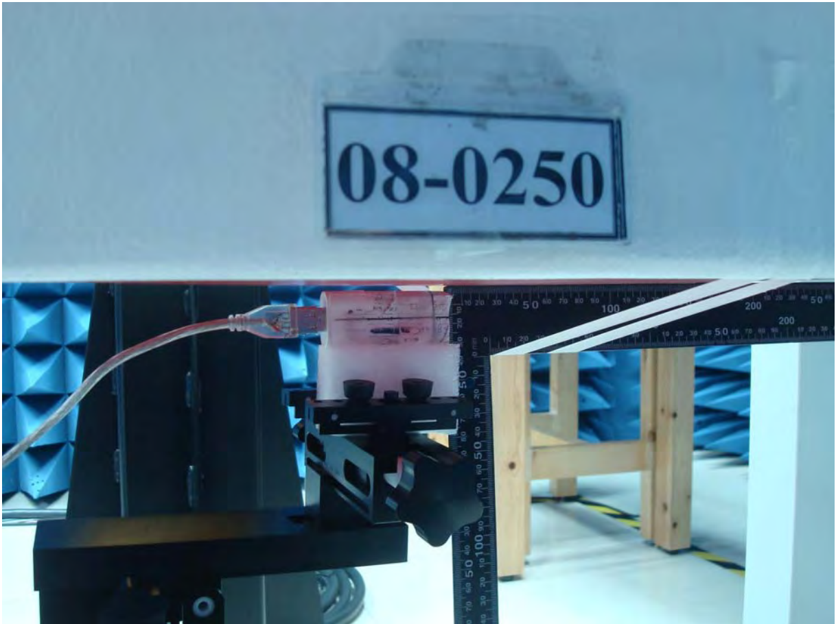
Figure 17. Body SAR Test Setup (Flat Section)
