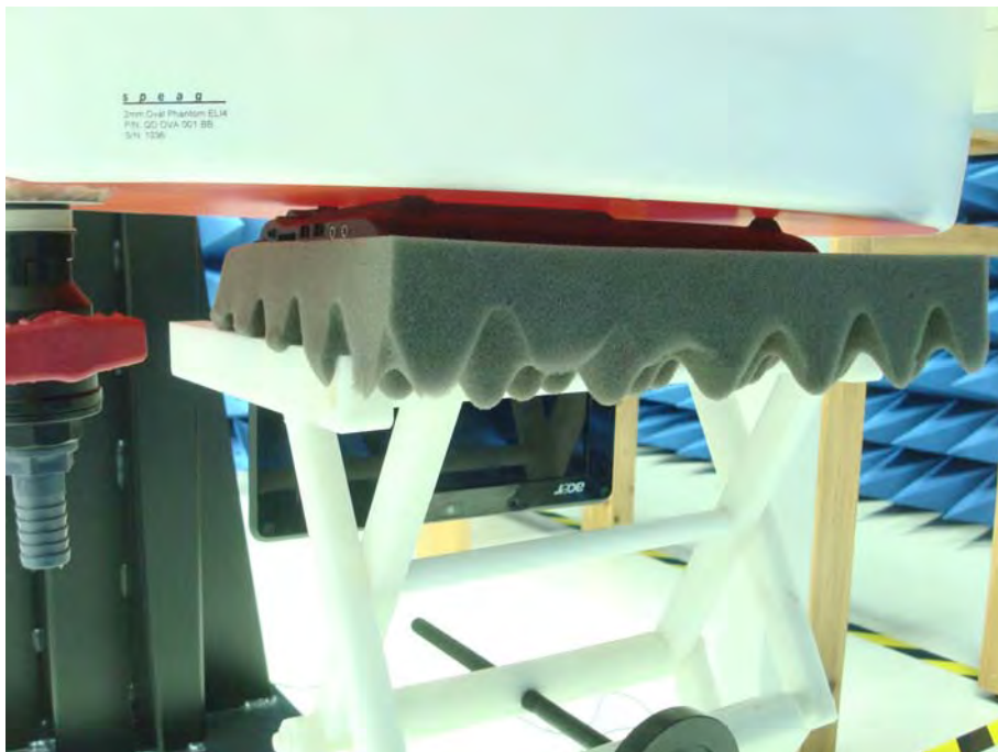
Figure 13. Laptop Holder with EUT
