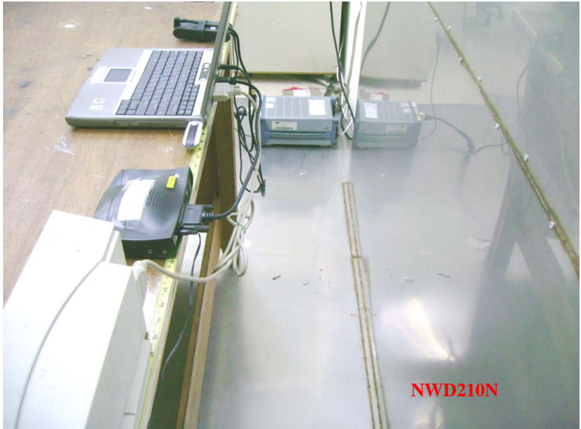
Photo 2: Conducted Emission Test Set-up photo
