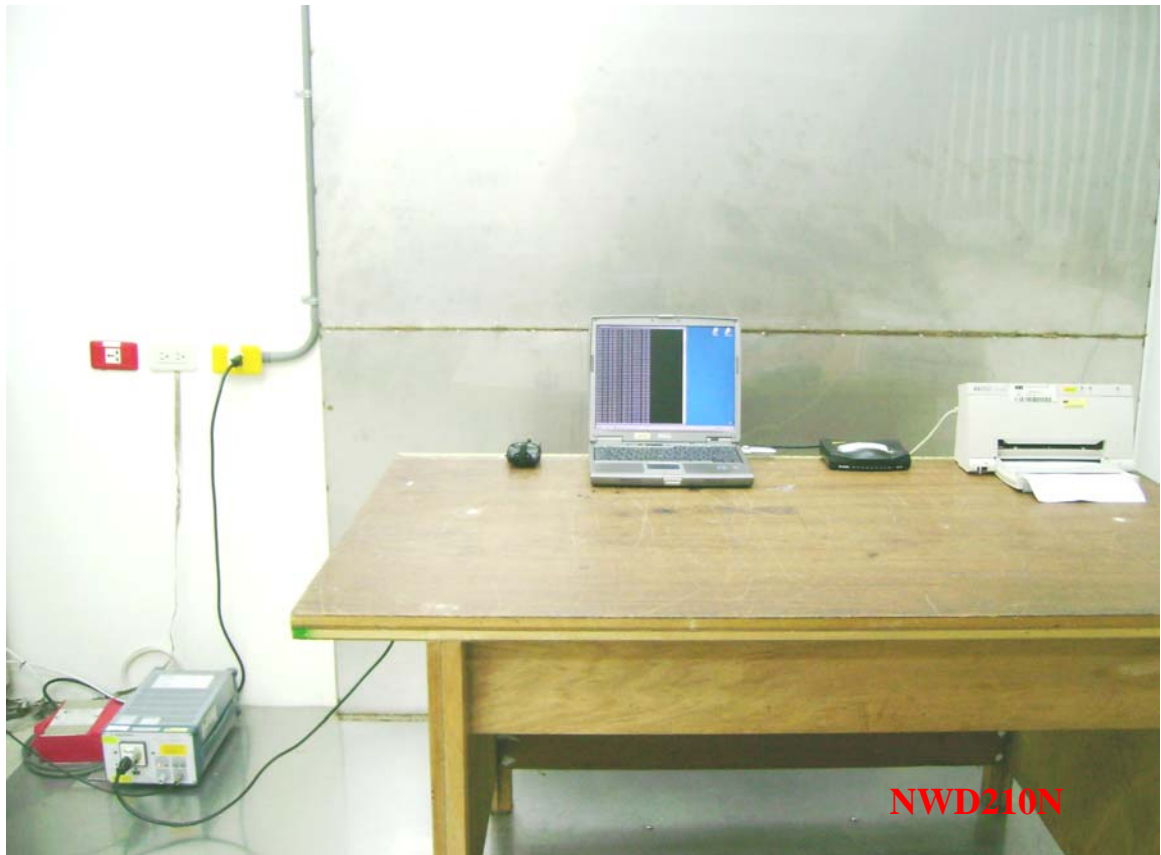
Photo 1: Conducted Emission Test Set-up photo
