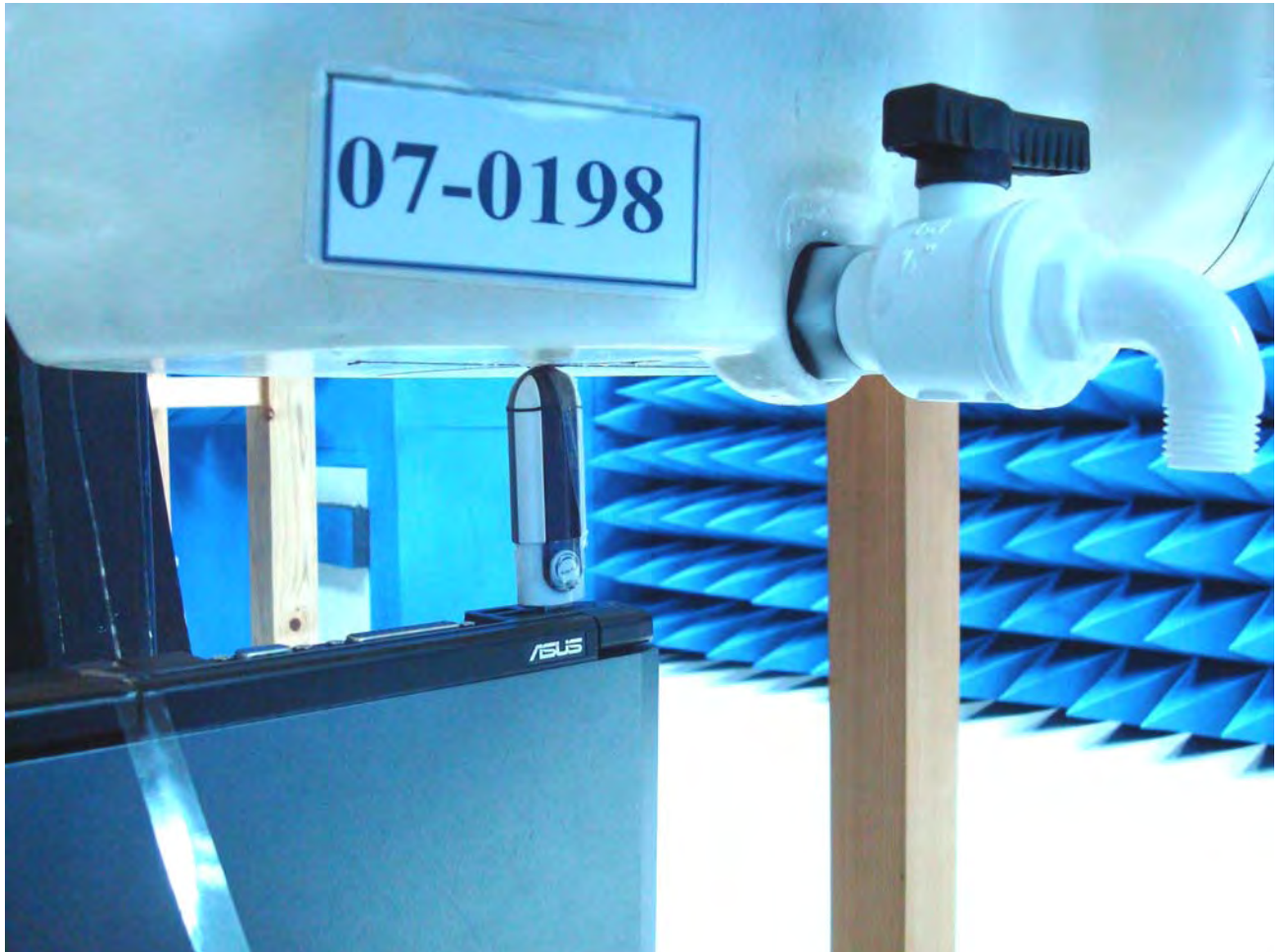
Figure 15.Body SAR Test Setup (Flat Section) _Top for NB No.2
