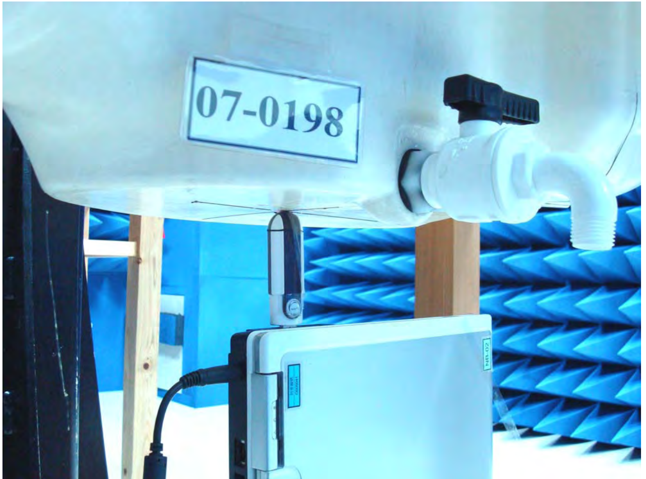
Figure 16. Body SAR Test Setup (Flat Section) _Top for NB No.3
