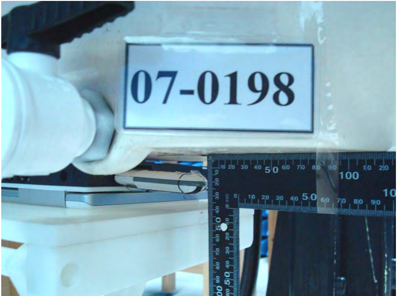
Figure 11.Body SAR Test Setup (Flat Section)_Bottom for NB No.1
