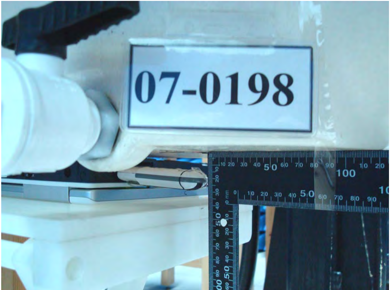
Figure 13. Body SAR Test Setup (Flat Section)_Bottom for NB No.3
