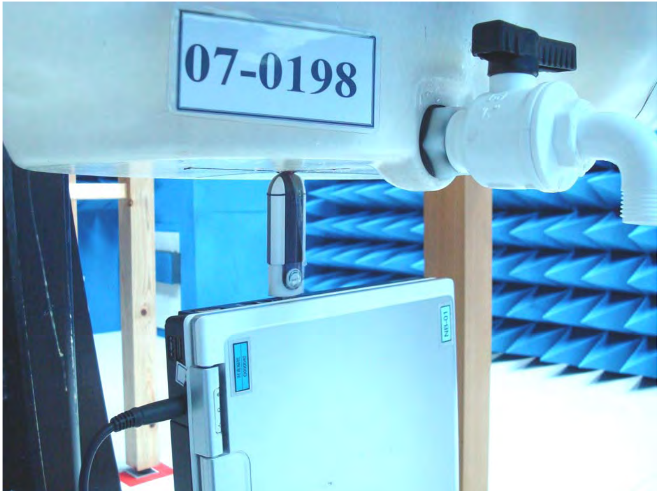
Figure 14. Body SAR Test Setup (Flat Section)_Top for NB No.1
