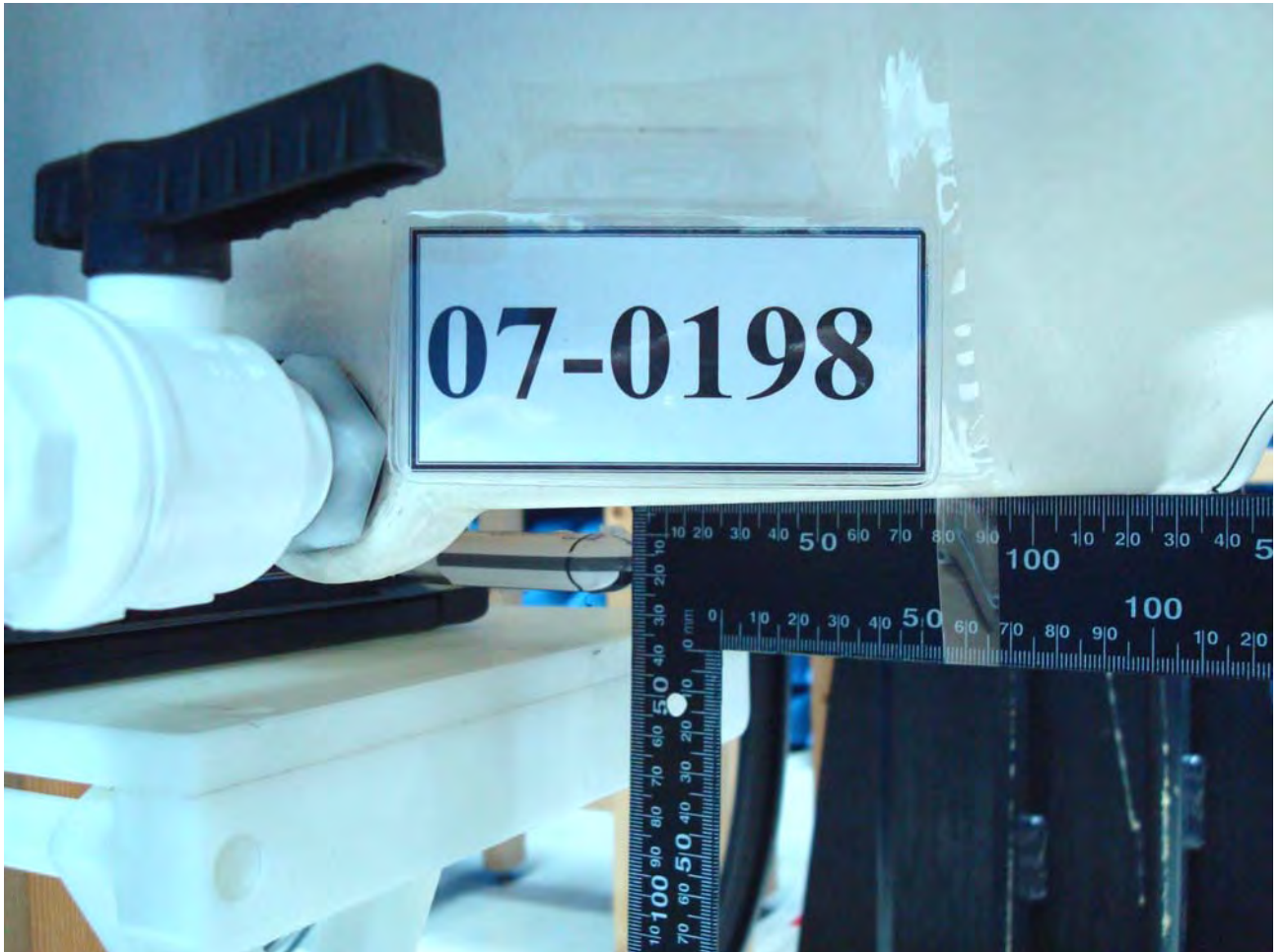
Figure 12. Body SAR Test Setup (Flat Section)_Bottom for NB No.2
