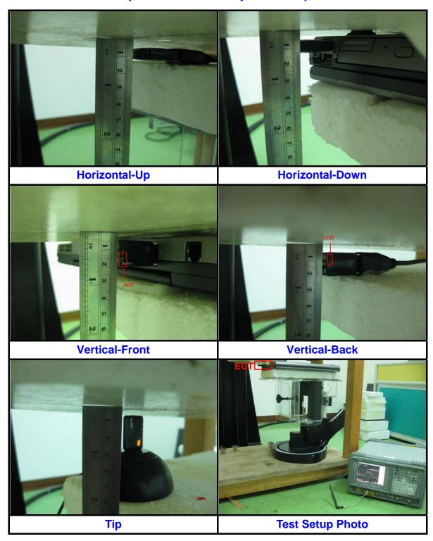
NOTE: The EUT face to the phantom with 5mm-separation distance.
