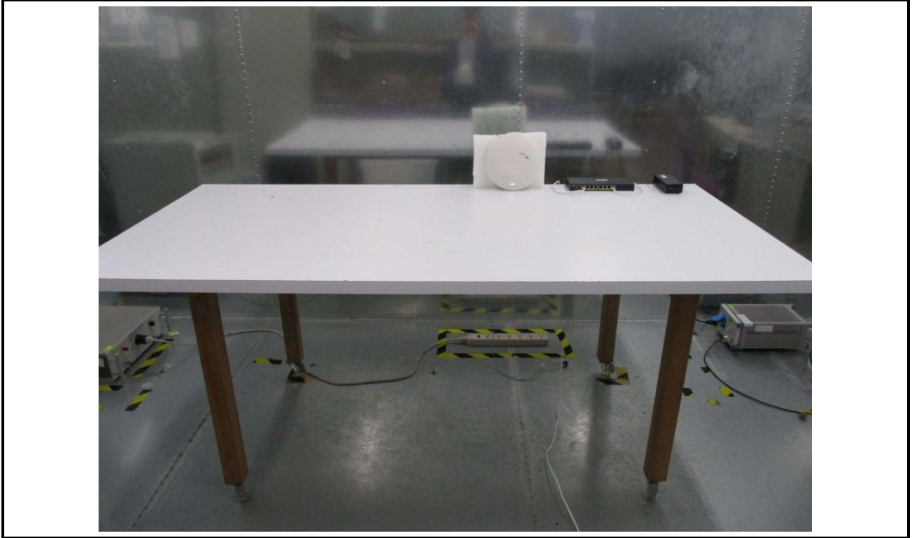
Conducted Emission Test (PoE mode)
