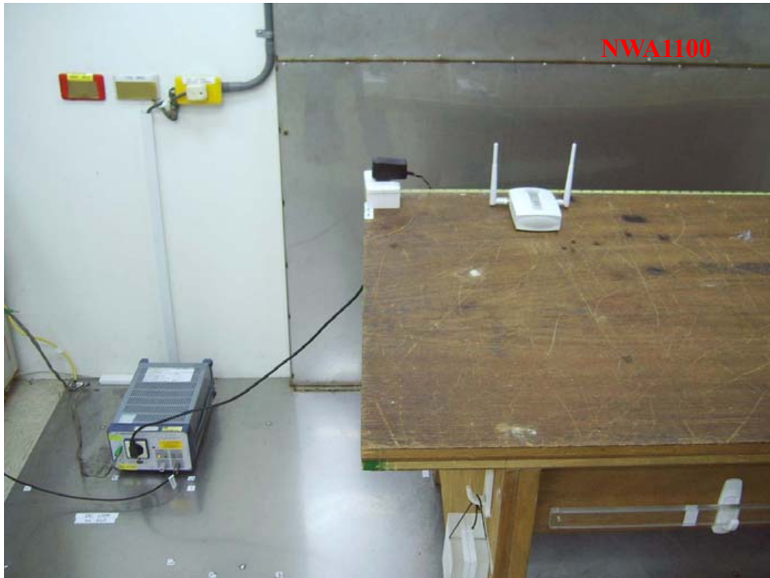
Photo 1: Conducted Emission Test Set-up photo
