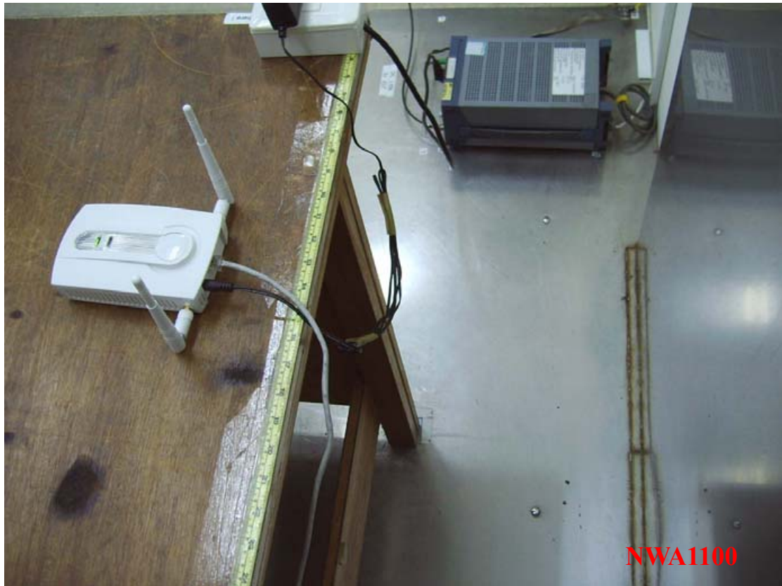
Photo 2: Conducted Emission Test Set-up photo
