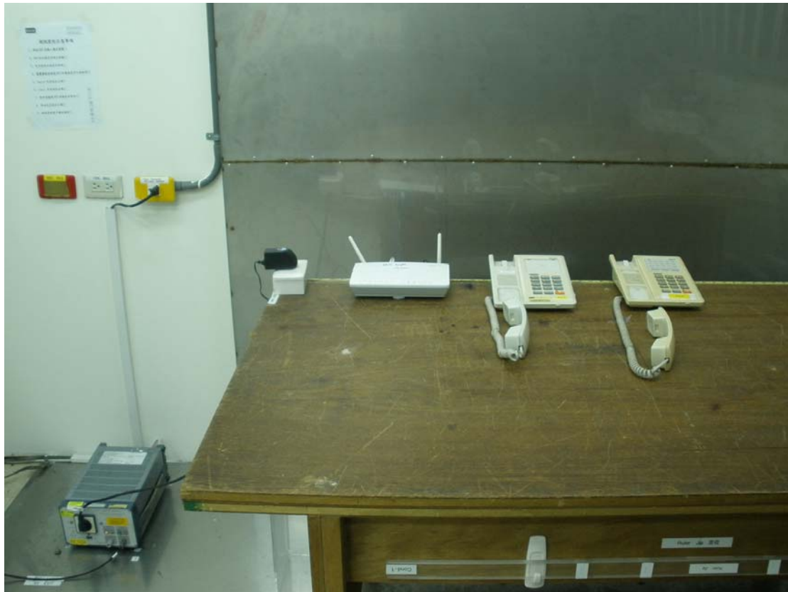
Photo 1: Conducted Emission Test Set-up photo
