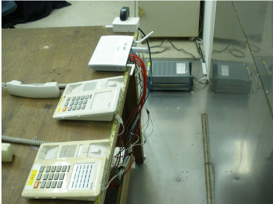
Photo 2: Conducted Emission Test Set-up photo
