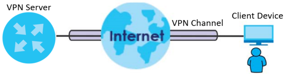
Figure 24 Example of NBG7815 Acting As VPN Server
