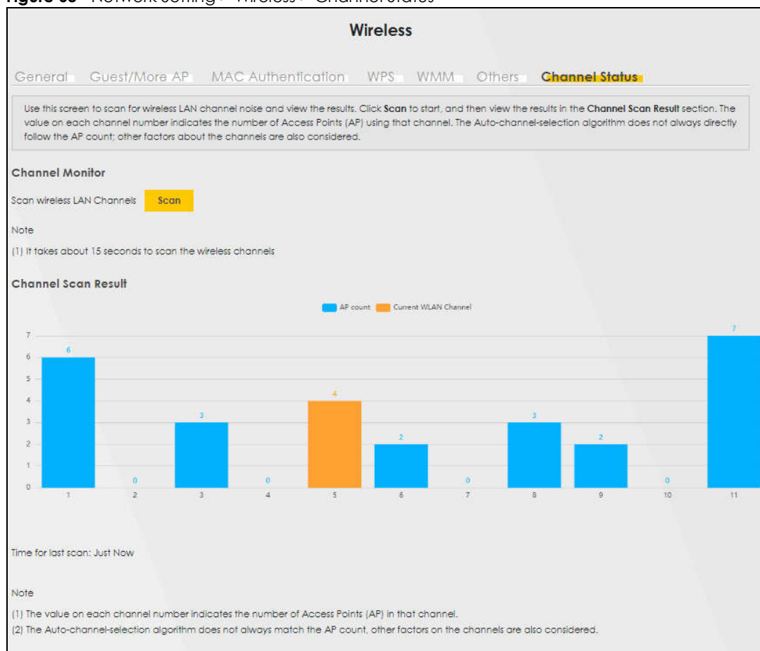
Figure 63 Network Setting > Wireless > Channel Status
