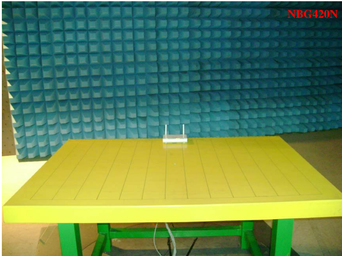
Photo 1: Radiated Emission Test set-up photo
