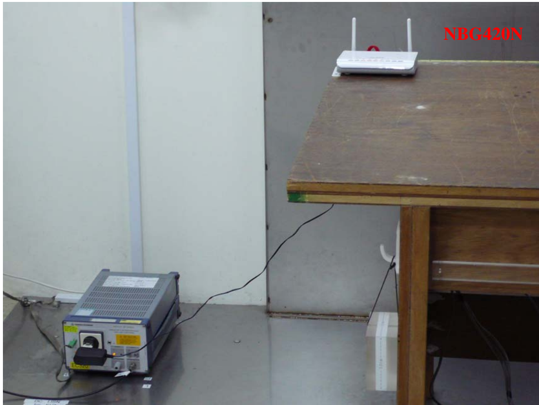
Photo 1: Conducted Emission Test Set-up photo
