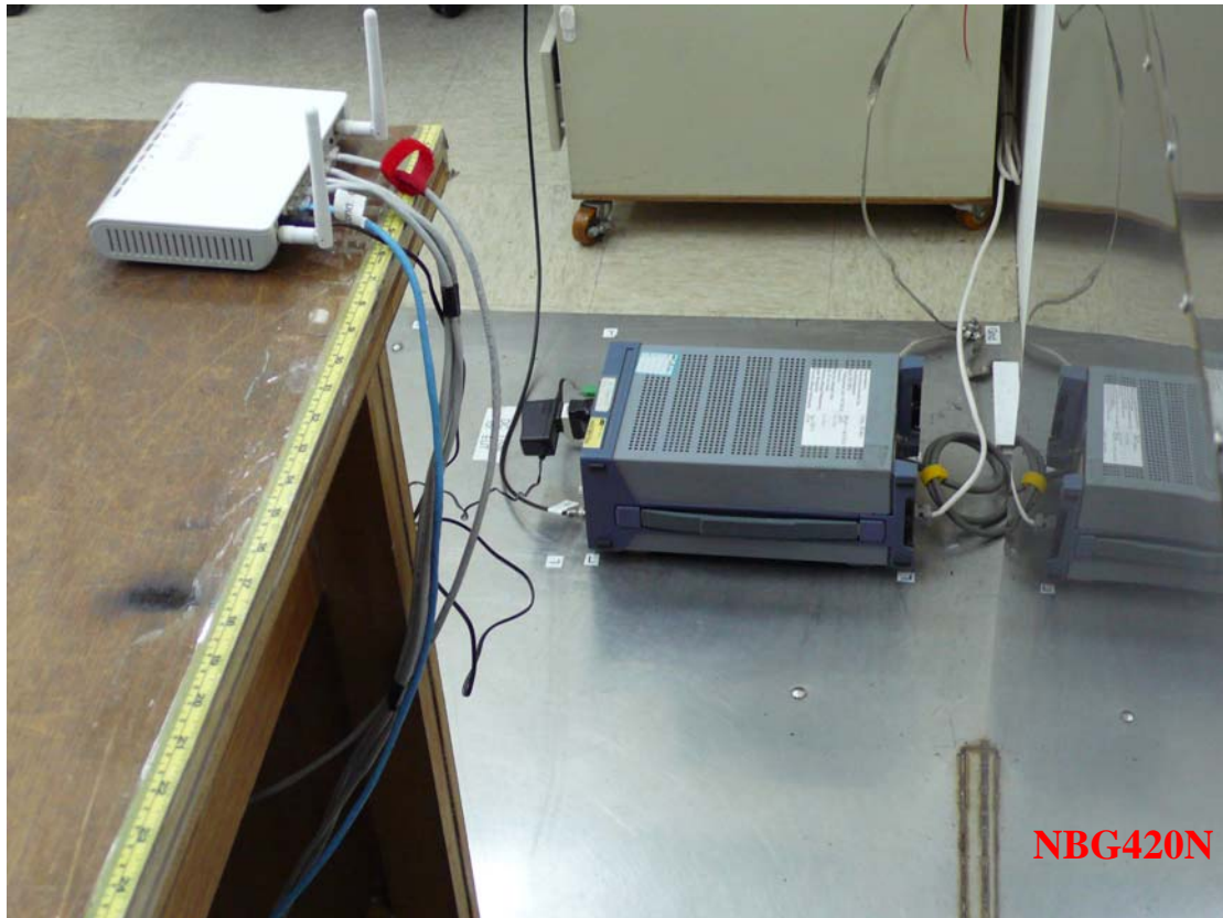
Photo 2: Conducted Emission Test Set-up photo
