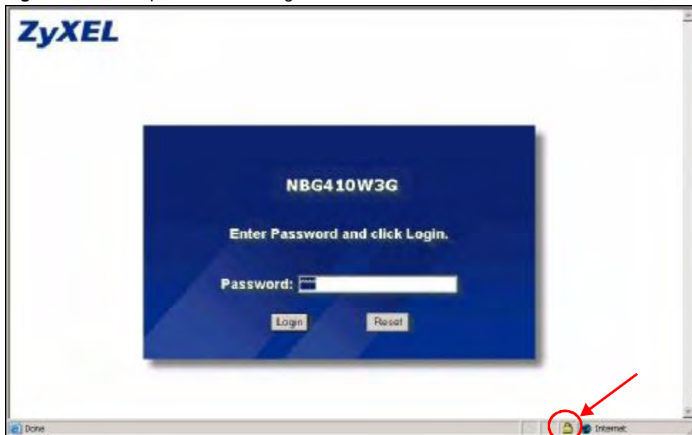
Figure 162 Example: Lock Denoting a Secure Connection
