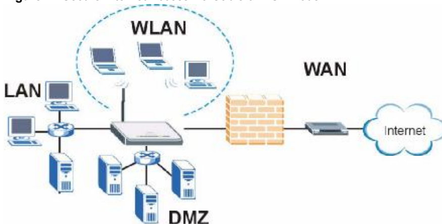
Figure 2 Secure Internet Access via Cable or DSL Modem
