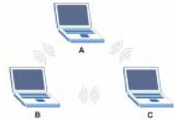
Figure 152 Peer-to-Peer Communication in an Ad-hoc Network
