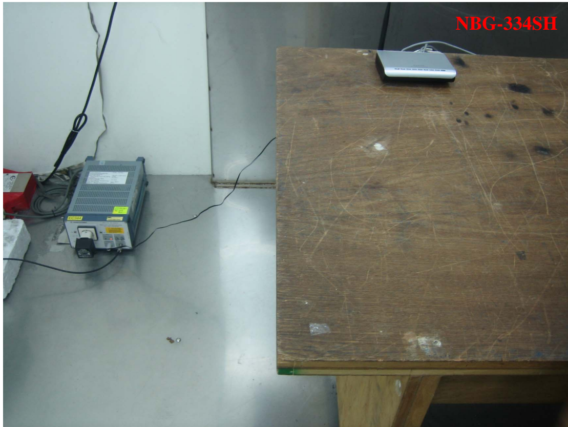
Photo 1: Conducted Emission Test Set-up photo
