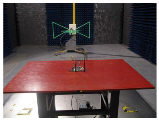
Test Mode : Mode 1~4: Transmit Description : Back View of Radiated Emission Test Setup for Under 1GHz
