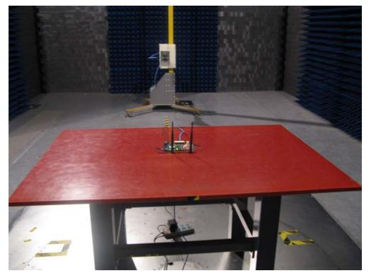
Test Mode : Mode 1~4: Transmit Description : Back View of Radiated Emission Test Setup for Above 1GHz
