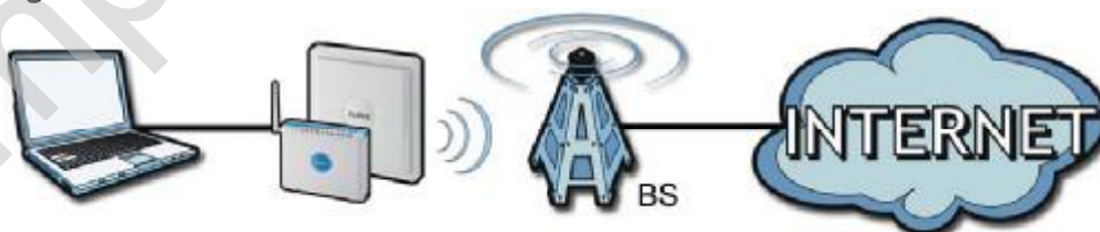
Figure 3 WiMAX Device and Base Station
