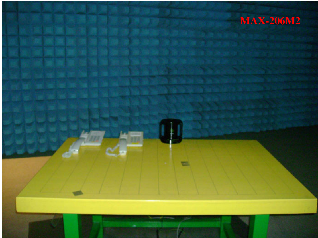
Photo 2: Radiated Emission Test set-up photo
