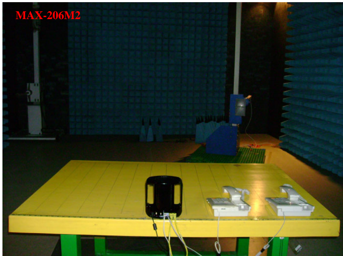
Photo 2: Radiated Emission Test set-up photo
