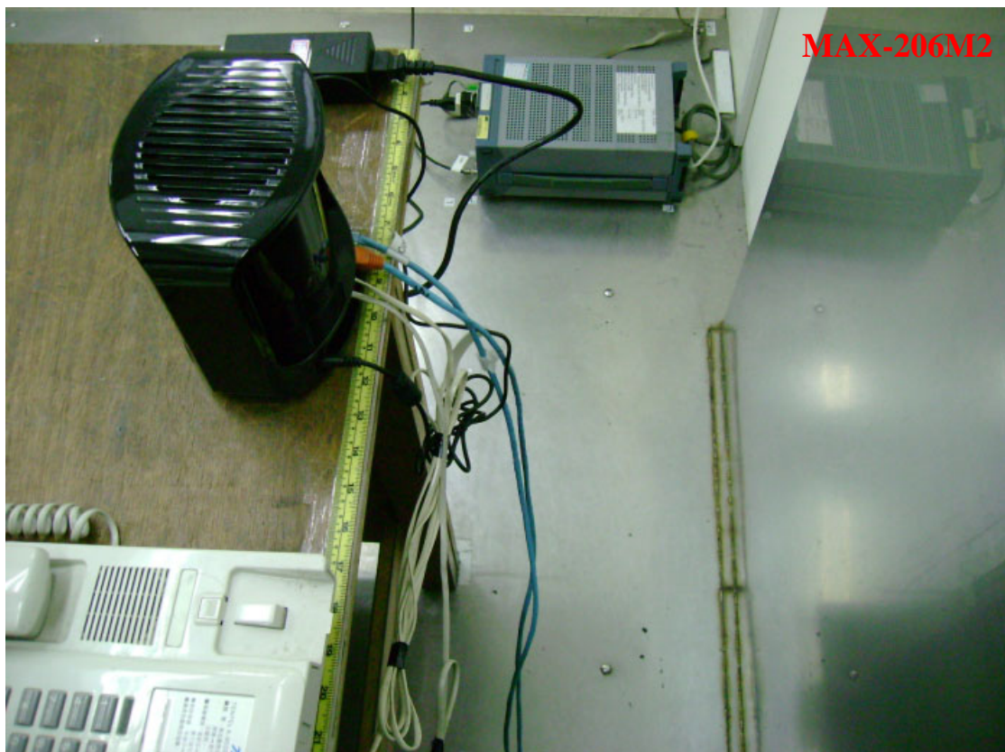
Photo 2: Conducted Emission Test Set-up photo
