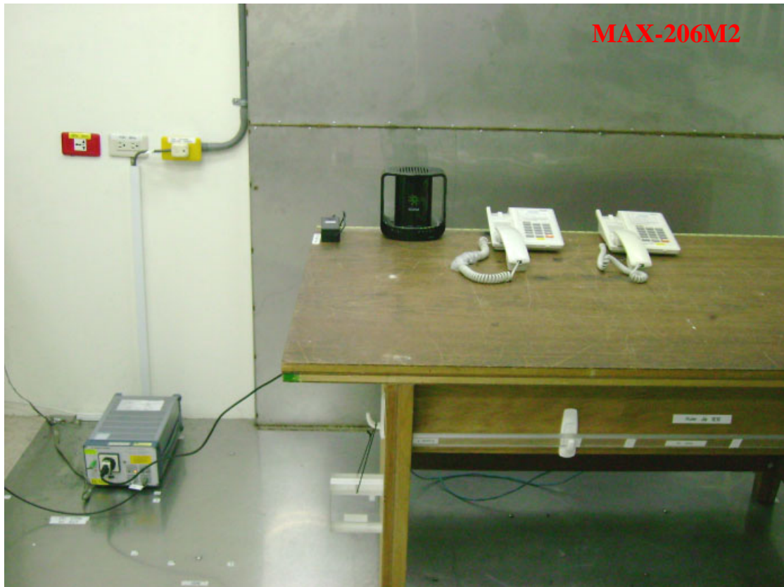
Photo 1: Conducted Emission Test Set-up photo
