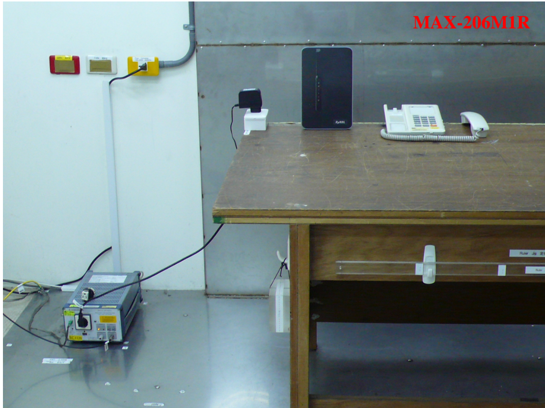
Photo 1: Conducted Emission Test Set-up photo
