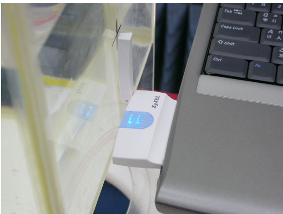
Figure 11: EUT perpendicular to phantom, 0 mm separation-Zoom in
