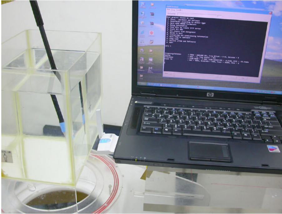
Figure 18: EUT perpendicular to phantom, 15 mm separation
