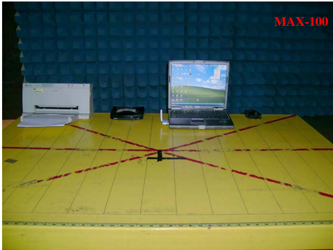
Photo 2: Radiated Emission Test set-up photo
