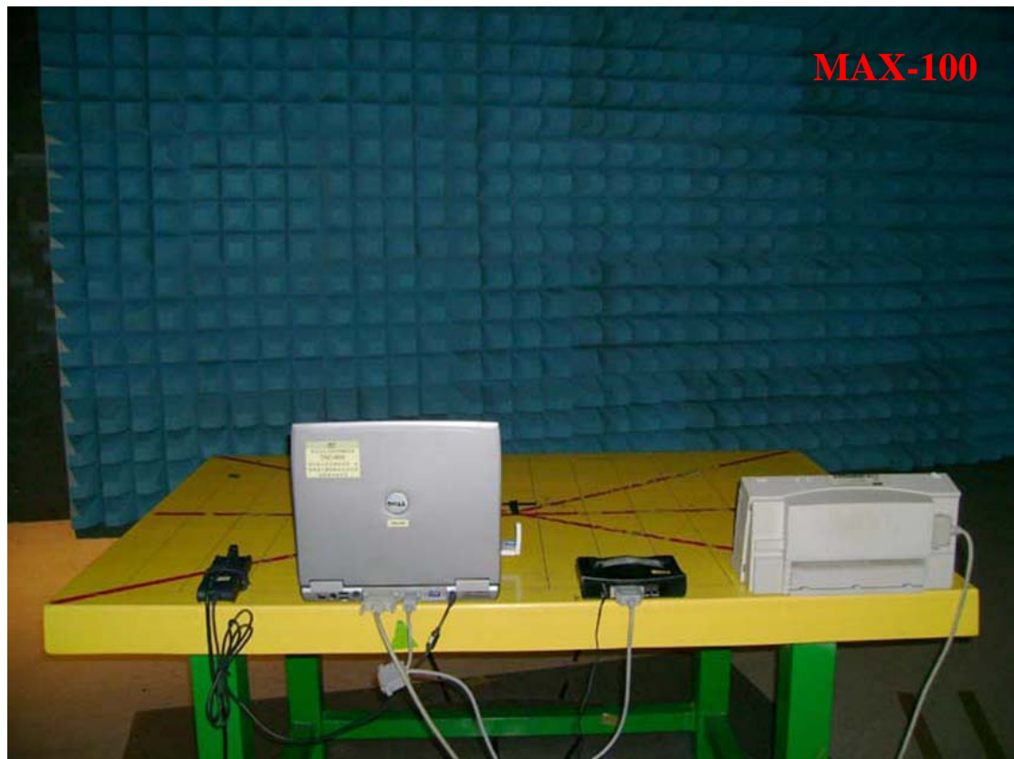
Photo 2: Radiated Emission Test set-up photo
